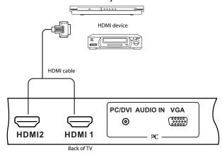
**Note:** To connect a DVI device, use a DVI to HDMI adapter cable to connect to the **HDMI** jack on the TV, then connect an audio cable to the **PC IN AUDIO** jack on the back of the TV.
